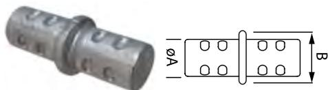
It provides a permanent in-line connection for 33.7mm diameter x 3.2mm thick tube. A crimping tool is necessary.
