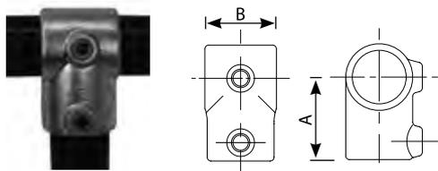
It provides a butt joint between two tubes at right angles to each other. Often used for railing ends and tops. If tubes need to be joined inside the fitting then a C04 type should be used.
