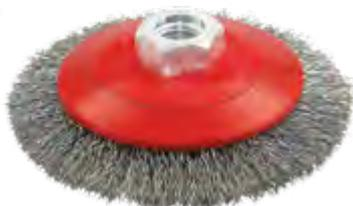
High tensile crimped steel wire, 0.3mm diameter, for rust and paint removal, descaling, deburring and preparation of welding seams. For metal and stone working, cleaning, surface preparation and fabrication tasks. Use with angle grinders.
