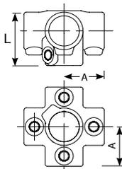
It provides a four way midrail joint for handrail and other structures. It is recommended that the handrail post is continuous through the fitting. This fitting may also be used for the top rail with the centre post capped with a C65 Plastic Stop End.
