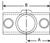
It provides the midrail joint for handrail and other structures. It is recommended that the handrail post is continuous through the fitting.
