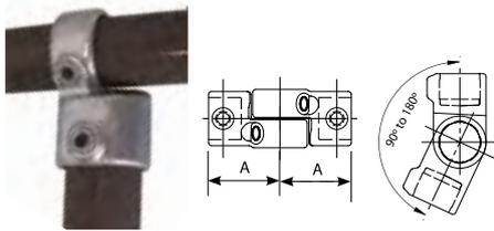
Short Tee Swivel fittings are normally used in pairs to facilitate corner angles of 90° to 180°. It is also used on staircases with a C02 and C03 fittings in conjunction with a short piece of tube and a C65 Plastic Stop End in landing areas.
