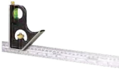
Combination square with metal body with three machined faces. The steel blade is stamped with metric and imperial sizes and is easy to read. Fitted with a 360° vial for all-round visibility and a scribe for convenience and marking out. Can be used as a try and mitre square, depth or height gauge and spirit level.
