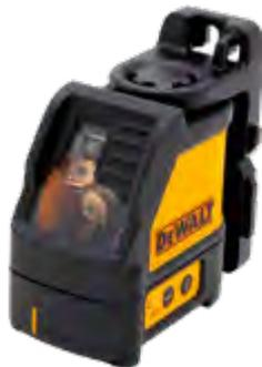
The DEWALT DW088K 2-Way Self-Levelling Line Laser is accurate to  $\pm 0.3\text{mm/m}$  in levelling applications. Self-levelling up to 4° surface angle with automatic out of level indication. It uses a simple 2 button operation with a low battery indication for ease of use.
