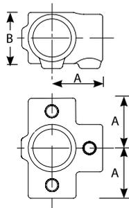
It provides a three way midrail joint for handrail and other structures. It is recommended that the handrail post is continuous through the fitting..
