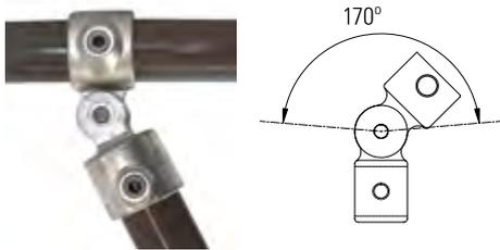
The Single Swivel Combination is designed to provide an angled tee between two tubes. It can be used to construct sloping handrails and for providing bracing struts to structures.
