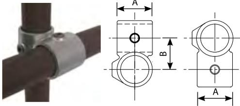
The 90° Crossover connects two rails at 90° to each other and is often used for the handrailing when continuous standard lengths of tube are used. Please note that tube joints should use the C00 or C01 type fitting, and not the C40 type fitting.
