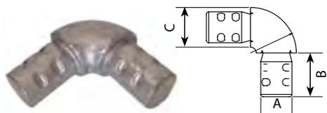
Crimp Elbow provides a permanent 90° connection for 33.7mm diameter x 3.2mm thick tube, a crimping tool is necessary.
