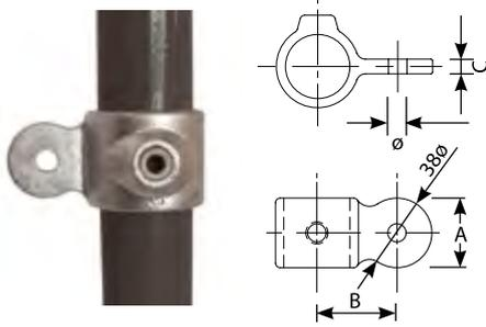
The Male Swivel can be used on its own for use with a shackle and chain or with the C36 female swivel to mount rails at any angle for slopes. It can also be used for attaching flat sheets or boards to a structure and is available assembled with the C36 fittings as a C45 single swivel combination.
