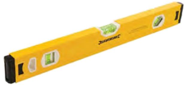
Extruded aluminium construction (1.1mm thick). Milled V-groove bottom face for accuracy and pipework applications. Ribbed sides, protective end caps and hanging hole. Highly visible, UV-resistant 45°, 90° and 180° vials. Accurate to 1mm/m.
