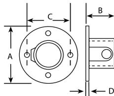
Designed to provide a positional wall or base fixing. It is not recommended to use this fitting as a structural railing base.
