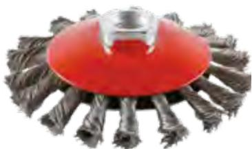
High tensile steel wire, 0.5mm diameter, for rust and paint removal, descaling, deburring and preparation of welding seams. For metal and stone working, cleaning, surface preparation and fabrication tasks. Use with angle grinders.
