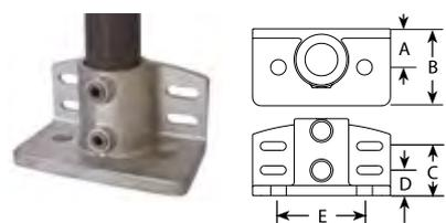
Ideal for guardrailing and balustrading applications where the addition of a toeboard is required. The side plates have slotted holes to allow for a degree of sideways movement for ease of installation.
