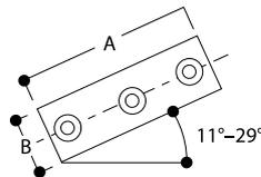
Similar to a type C26, it is used on safety railing with slopes between 11°-30° and fixes the mid rail to a vertical intermediate upright. Unlike the type C26 these components are ex-stock and do not require machining.
