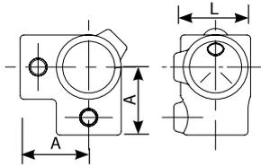
The Corner complete with through tube is designed to provide a 90° corner for the intermediate rail of guardrail or frames.
