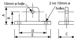
The Swivel Base is designed to provide a base fixing. It is usually used in conjunction with a C36 type fitting to make a C46 type base swivel combination. This fitting does not provide sufficient rigidity to be used as a railing base without other means of support.
