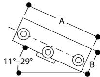
Similar to a type C27, it is used on safety railing with slopes between 11°-30° and fixes the top rail to a vertical intermediate upright. Unlike the type C27 these components are ex-stock and do not require machining.
