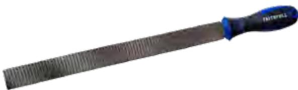
The Faithfull flat wood rasp is for use on wood or soft metals, for professional or frequent DIY use. This range of rasps has coarse bastard teeth with single cut edges and is fitted with a comfortable handle. Blade width 27mm
