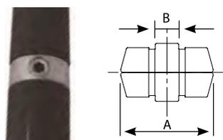
Providing an in line joint between tubes of the same diameter, and a wall thickness of 3.2mm. It fits flush with the tube surface and can be located inside other fittings. It must not be used as a load-bearing joint, in these applications use a FastClamp type C00.
