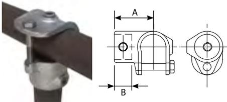
The Clamp on Tee is designed to allow a new tube to be joined to an existing structure. Torque maximum 15Nm. This uses an M10 stainless steel bolt.
