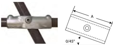
Typically used for guardrail when connecting the mid or lower rails to uprights. The upright tube must remain continuous with the mid and lower rails cut to suit. The C26 is normally used in conjunction with a C27. Fittings are stocked as blanks and are machined to the customer's specified angle between 0° and 45°.
