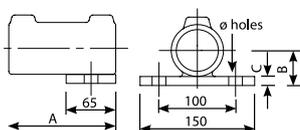
It provides a base for railings and other structures that need a side mounted fixing.
