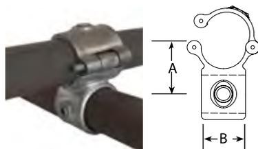
It allows existing structures to be added to without the need for any dismantling. This fitting is designed to give a 90° offset crossover joint. Tubes must not be joined within this fitting.
