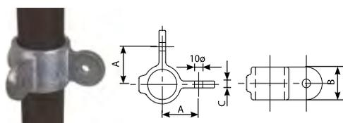
The 90° Corner Male Swivel is designed as part of the swivel combination group of fittings. It can be used with two C36 female swivel fittings to make a corner combination fitting which is also available assembled as a type C48 fitting.
