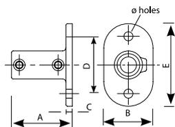
It provides a positional wall or base fixing. It is not recommended to use this fitting as a structural railing base.
