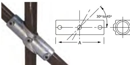
The Adjustable 2 Socket Cross fitting will accommodate any rake angle from 30° to 45°. This fitting is not recommended as the top fitting on a guardrail or balustrade system, use the C29 Adjustable Short Tee.
