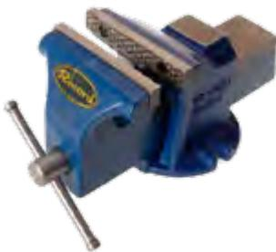
The IRWIN® Record® Pro Entry Mechanic's Vice is fully machined on all load bearing surfaces for smooth and trouble free operation. It features a safety stop to prevent the slide being separated from body and a fused handle, Acme twin start thread for smooth and fast operation and replaceable hardened steel jaws (55 HRC).
