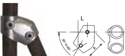
It will accommodate any rake angle from 30° to 60°. Commonly used for the top rail of handrail to accommodate the rake angle on slopes, it can also be used for any Tee Joint that needs to make at an angle of between 30° and 60° for lightweight structures.
