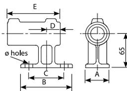
The Railing Vertical Side Support is designed to provide a base for railings and other structures that need a side mounted fixing.
